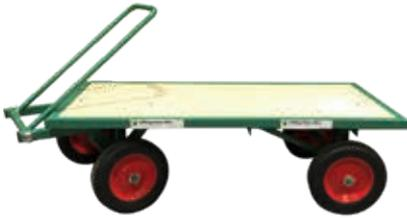
Heavy duty turntable truck capable of holding up to 1000kg. Featuring an 18mm plywood base. Supported by box section and steel angle with solid wheels.
